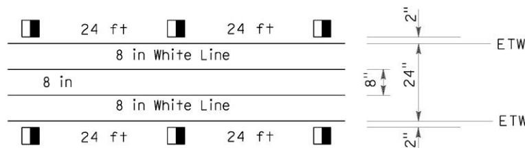
Source: CAMUTCD, Striping Detail 44 with 8-Inch Separation and Channelizers for a 2-Foot Buffer
